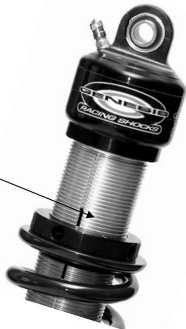
All Genesis aluminum shock bodies have two grooves 180° apart. The coil-over adjusting nuts also have two grooves 180° apart. By lining up the grooves and inserting a tie-strap, the nut is locked in place.
